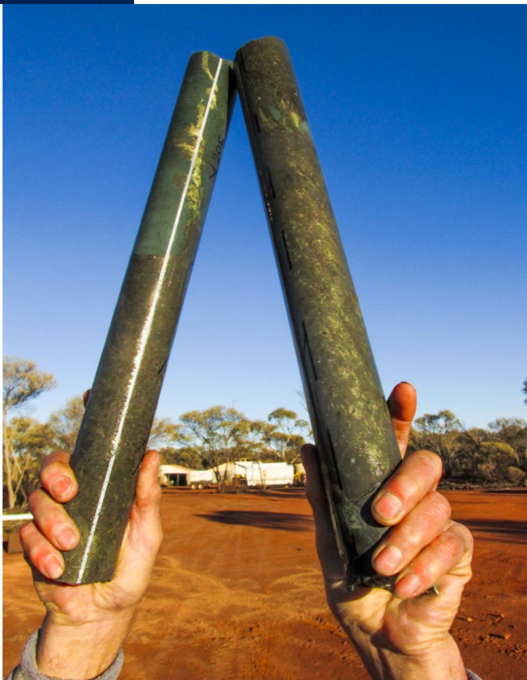
Figure 4: 70cm intersection of massive sulphide in DKDD0017 with the Rosie Camp in the background
