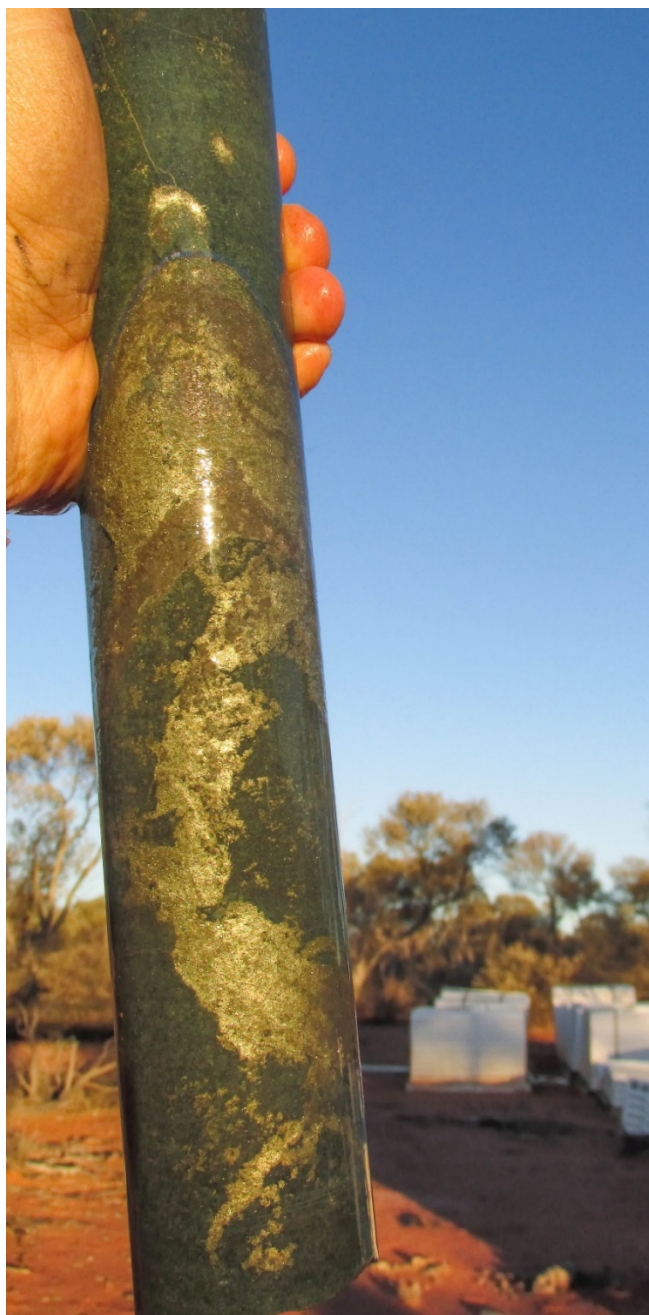
Figure 5: Pentlandite rich stringer sulphides in drillhole DKDD0017
